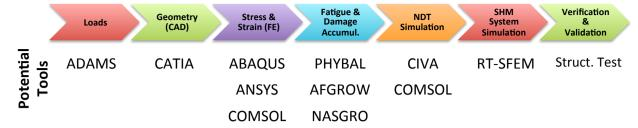
We simulate stresses, strains, damage and even the monitoring systems for complex shaped and fatigue loaded structures
